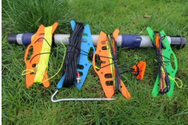
Figure 2, Linked dipole (615g) and 10m telescopic mast (1.3kg).
