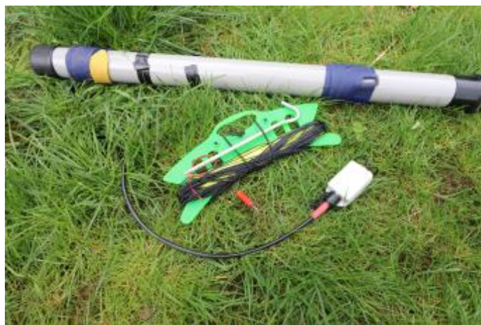
Figure 3, EFHW (245g) and 10m telescopic mast (1.3kg).
